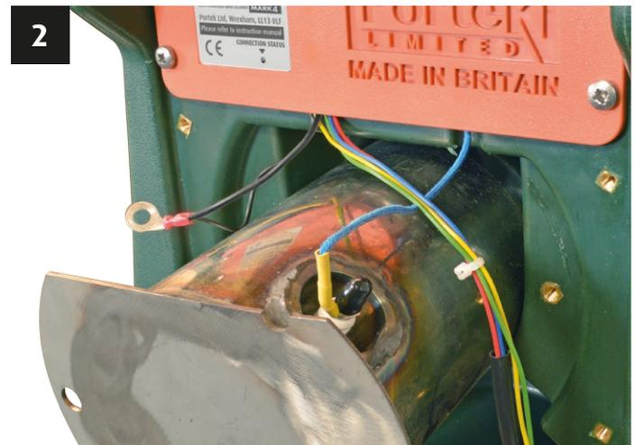
8. **Spark plug:** If the unit does not bang, then it could be that the spark is not igniting the gas. Check the High Tension (HT) lead from the spark generator is in good condition. To gain access to the spark plug the metal barrel needs to be partly removed from the main housing.
