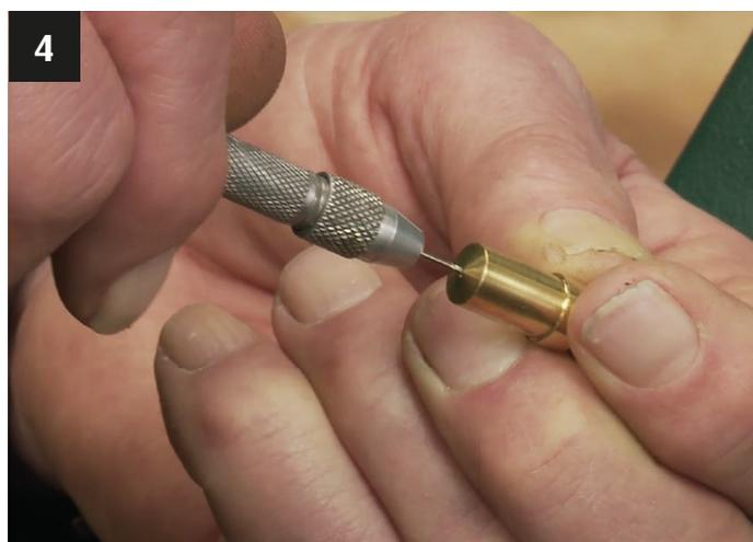
7. **Cleaning the gas jet:** If the unit goes bang but is erratic (perhaps banging 3 out of the 4 times or 2 out of 5 for instance) then this is most likely due to insufficient gas being delivered each time and the gas jet could be partially blocked.
